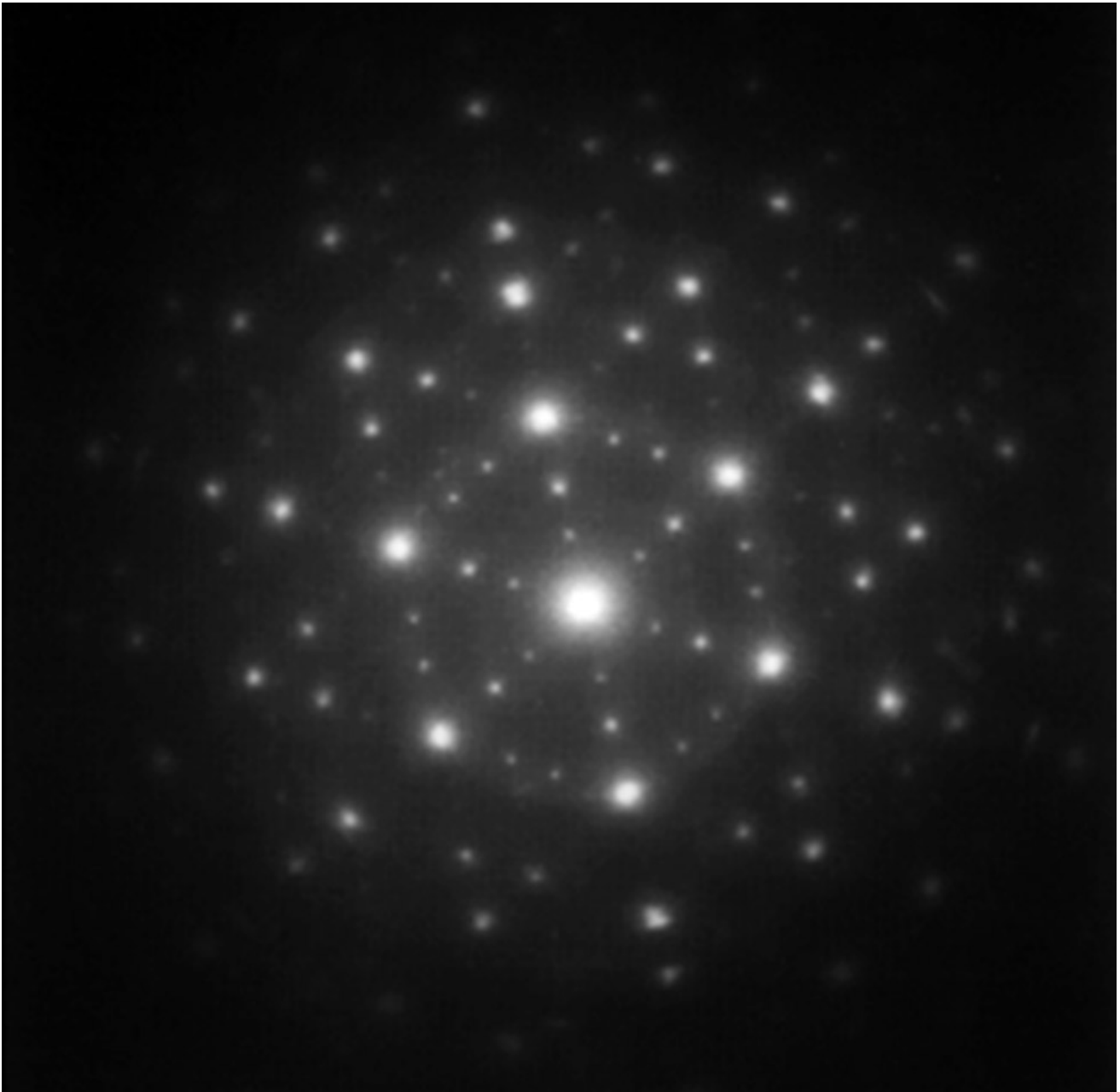
Selected area diffraction pattern of quasicrystals in a magnesium alloy. Image courtesy Julie Cairney, University of Sydney.
